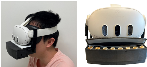
Figure 4: Wearable olfactory display beneath an HMD. The front lid can be open when the olfactory display is attached to the HMD, and it can be closed by the embedded magnets.
