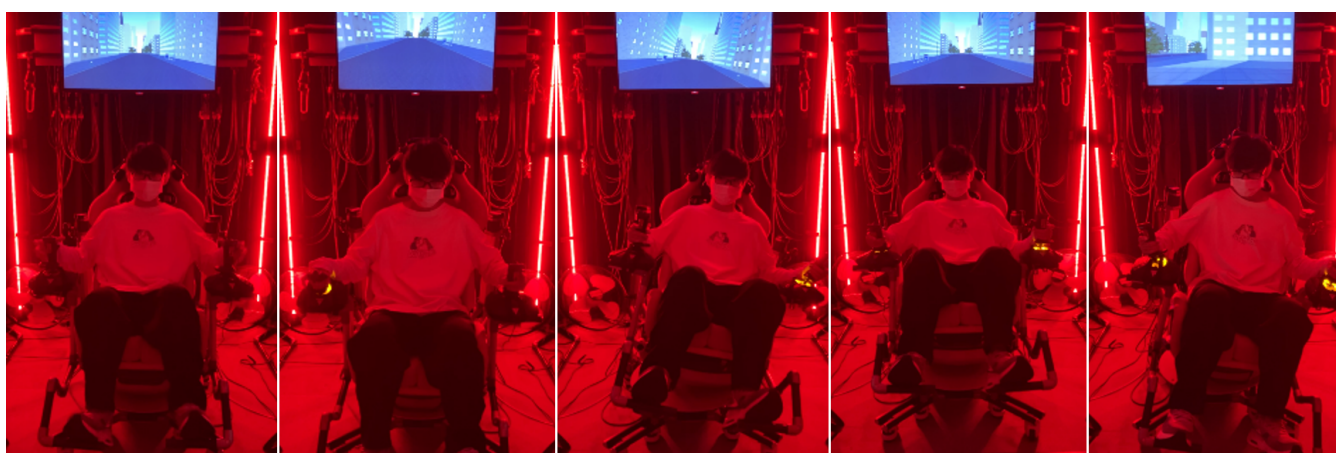
Figure 1: Pseudo 6-axis Motion Rendering results. From left: neutral, posture (pitch and roll), and inertia (surge and sway).
