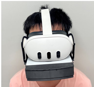
Figure 8: The olfactory display integrated with an HMD. The external air pump and deodorant filter are not shown here.
